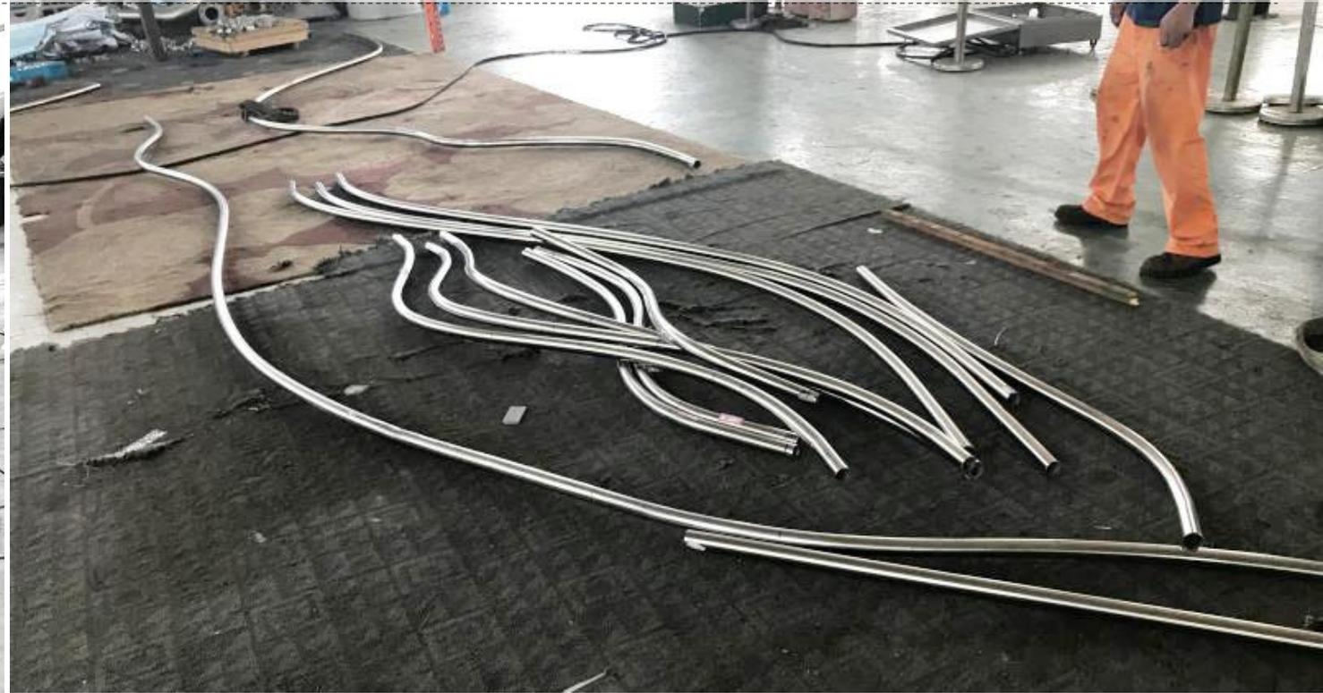
All the members have been optimized with some custom scripts to ensure they can be fabricated from a series of tangent arcs segments. A tolerance of 10mm deviation from initial architect geometry has been setup and the script find by itself the best fitting geometry. The complete structure has been preassembled in factory to ensure the fit and fabrication precision.
