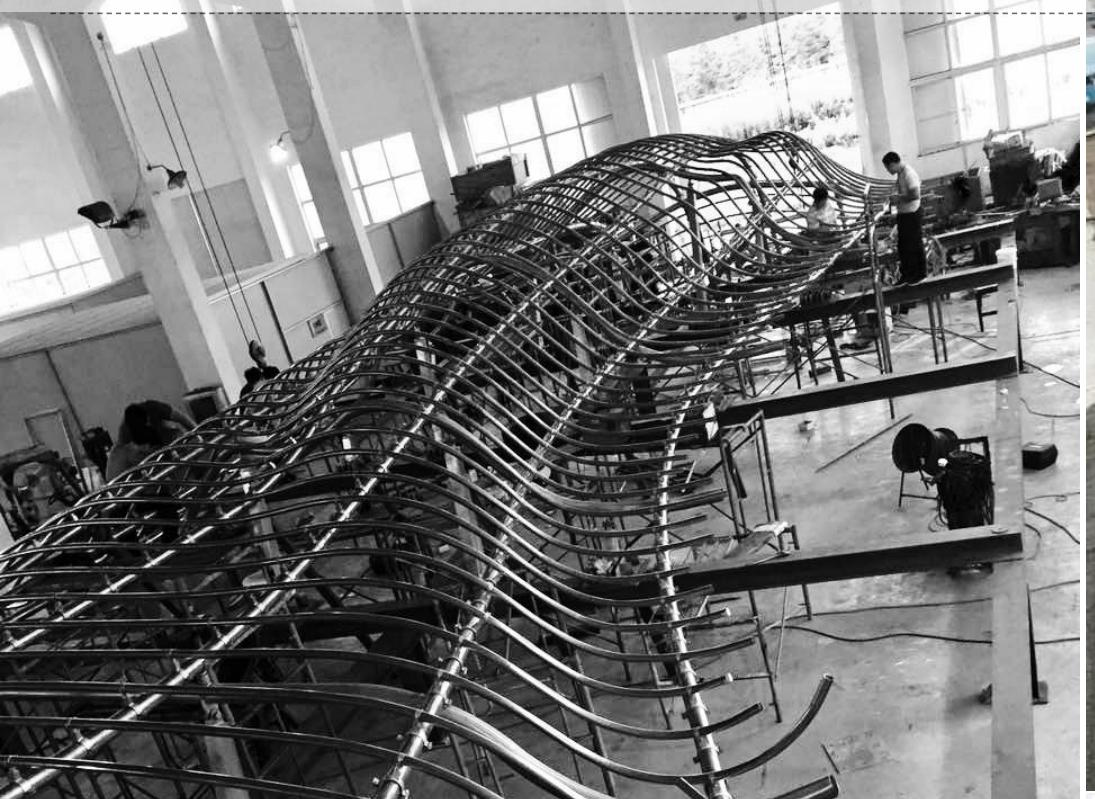
All the members have been optimized with some custom scripts to ensure they can be fabricated from a series of tangent arcs segments. A tolerance of 10mm deviation from initial architect geometry has been setup and the script find by itself the best fitting geometry.
